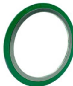
Spiral wound gaskets are manufactured by winding preformed metal strip and a soft filler material into a spiral seal with excellent mechanical resistance and recovery. They are available with or without retaining rings, and in a wide range of materials to ensure compatibility with the sealing media and operating conditions.
