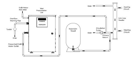
Please note that for the purpose of clarity, system valves are not shown. The expansion vessel should be installed in the most neutral point in the system regarding pressure and temperature. For systems exceeding 90°C contact our helpline for advice.
