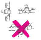
The valve can be installed in both horizontal and vertical pipes.
